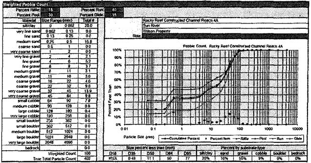
Figure 7. Weighted and Component Pebble Counts, Existing Condition
