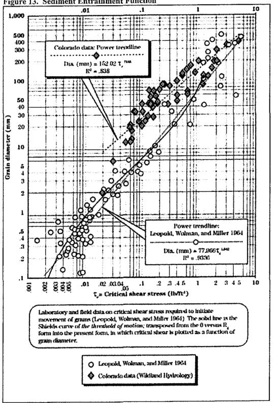
Figure 13. Sediment Entrainment Function
