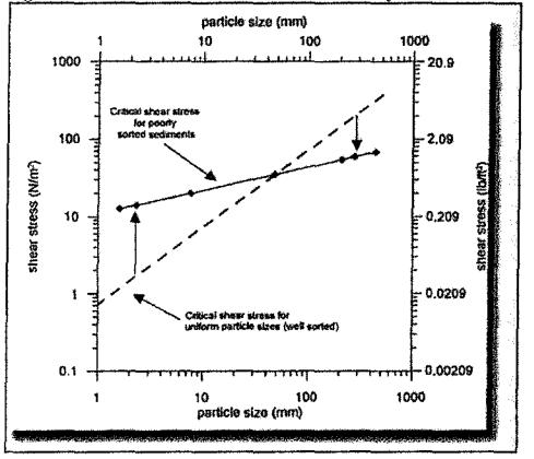
Figure 14. Shear Stress vs. Entrainment for Poorly Sorted Bed Material
